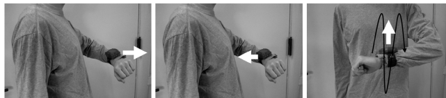
Fig. 2. Gestures used to operate the eWatch device: “scroll-up”, “scroll-down”, and “select”
