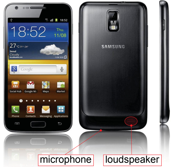
Figure 2: Samsung Galaxy SII smartphone used during the evaluation study. The distance between loudspeaker and microphone was 2.4 cm.
