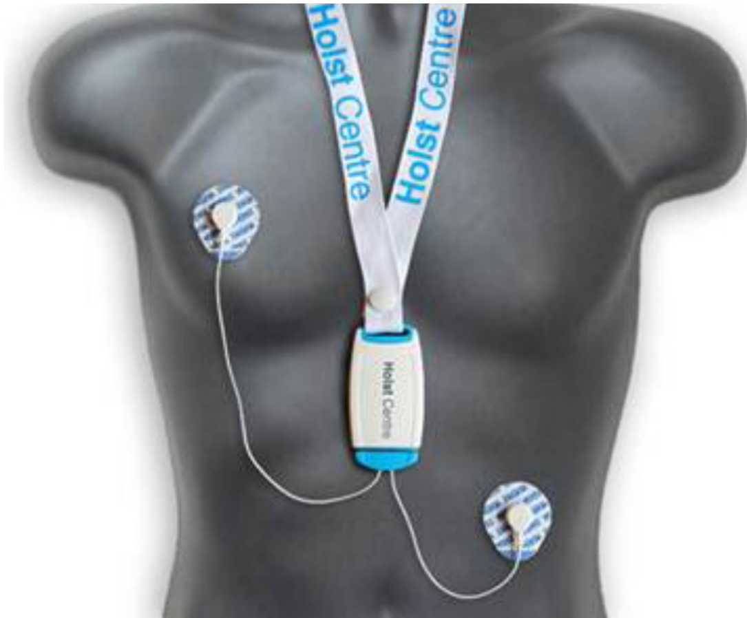
Figure 2. ECG Necklace. The device was used to acquire ECG and accelerometer data.
