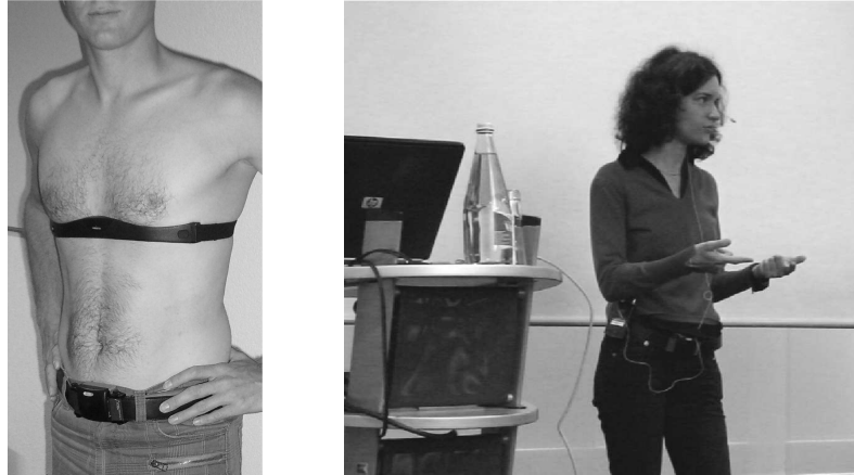
Fig. 3. Wearable system used for the recording of heart period data during the conference session. Left: Heart monitor belt attached to the thorax and QBIC belt computer for data storage. Right: Speaker wearing the system during the conference talk.
