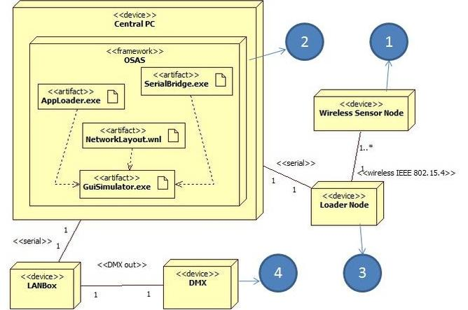
Fig. 9. Deployment view of the system architecture.
