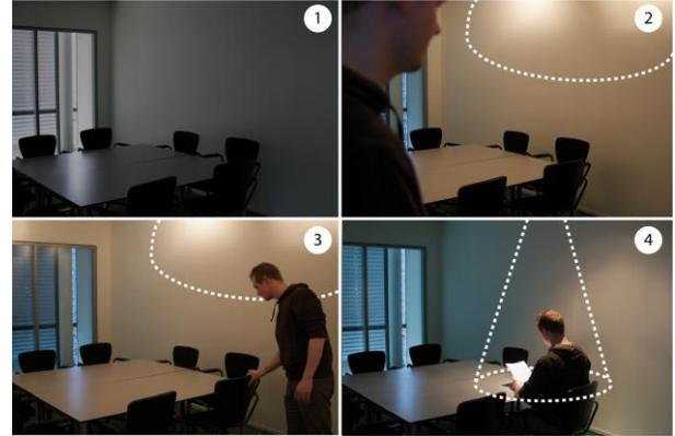
Fig. 3. Individual Scenario. When the user enters the room (1), general illumination is provided (2). When the user sits down, a spotlight on his task area is provided. The dotted lines illustrates the location of the lighting.
