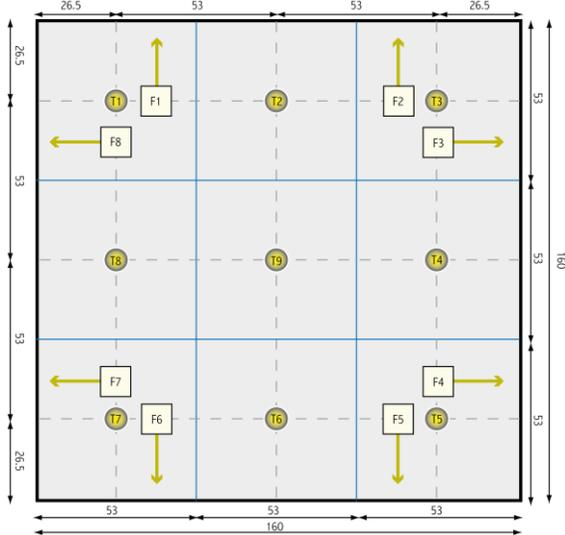
Fig. 2. Bottom view of custom ceiling design. The blue lines show the size of the tiles. The circles at the center of each tile represent the Task lights (T), directed downward. The square forms show the position of the Face lights (F) aimed at people. The arrow indicates the direction in which the Face light is aimed. All lights are counted from the top-left clockwise inwards. Environment lights are not visible in this image.
