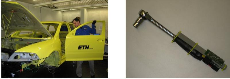
**Fig. 3.** Left: worker mounting the front door of the car. Right: socket wrench equipped with acceleration sensing wireless nodes.
