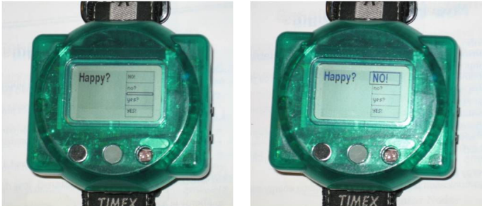
Fig. 1. Questionnaire application running on the eWatch. Left: Initial state, right: state after scrolling up.
