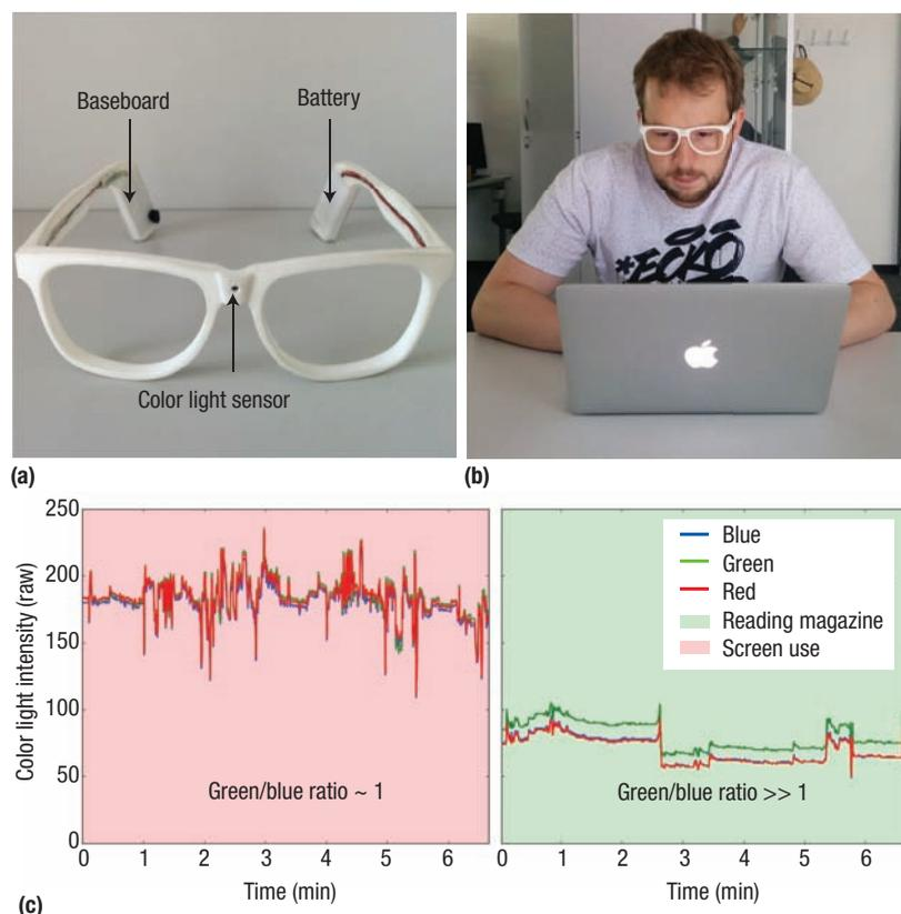
**FIGURE 3.** Screen-use detection with smart eyeglasses. (a) Smart eyeglass components for screen-use detection. (b) Participant wearing smart eyeglasses while performing activities. (c) Example light intensity data for red, green, and blue color channels while using a screen and reading a print magazine. Ratios of color channels clearly differ between activities.
