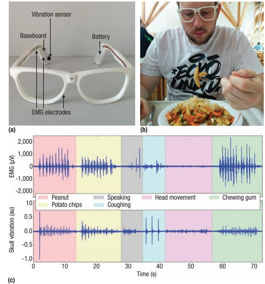
**FIGURE 4.** Nutrition monitoring with smart eyeglasses. (a) Smart eyeglasses components used to monitor chewing. (b) Participant wearing smart eyeglasses in daily life. (c) Example surface electromyography (EMG) and skull vibration data during a series of chewing and non-chewing activities. Signal patterns differ among activities.
