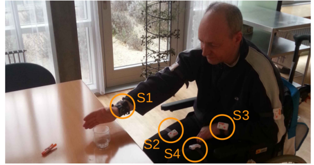
Figure 1. Patient at the day-care centre wearing the sensor setup while performing a drinking gesture. Sensor positions at the wrist and upper leg are indicated (S1, ..., S4).
