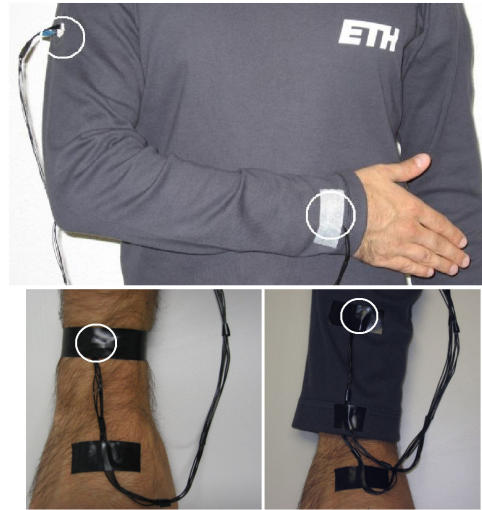
Fig. 4. Upper plot: placement of acceleration sensors on right lower and upper arm. Lower plot: skin- and garment-attached acceleration sensors at the right wrist (sensor-positions marked with circles).
