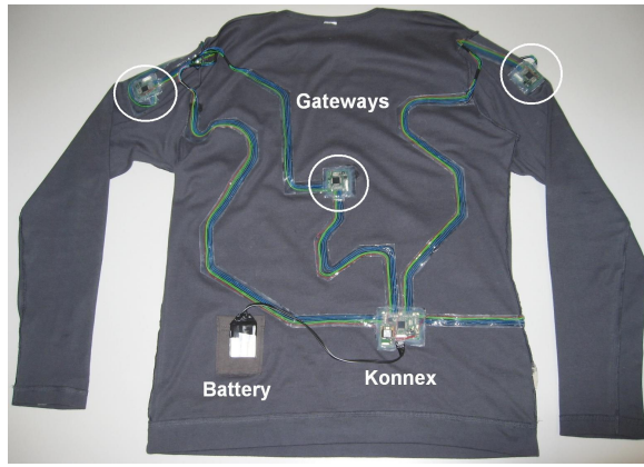
Fig. 1. SMASH system (inner side) with the Konnex and three Gateways (marked with a circle). The fourth Gateway is hidden.
