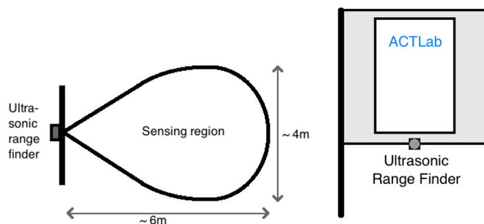
**Fig. 1.** On the left, a top view of a poster is given and the sensing region of the sensor is indicated. The exact shape of the sensing area depends on the sensor type. On the right it is shown how the ultrasonic range finder is positioned near a poster.
