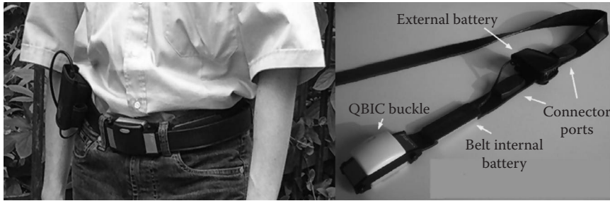
FIGURE 22.5 Example of accessory-based wearable computer: QBIC belt-integrated computer and system schematic. (From Amft, O. et al., Design of the QBIC wearable computing platform, Proceedings of 15th IEEE International Conference on Application-Specific Systems, Architectures, and Processors (ASAP) , Galveston, TX, 2004, pp. 398–410.)
