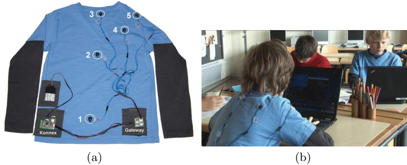
Fig. 2. (a) Sensing garment based on the SMASH architecture used in monitoring spine inclination in children. Five acceleration sensors were attached to the shirts using silicone gel (encircled positions) [4]. (b) Children wearing the garments in their school class. Inappropriate sitting habits could be improved by providing reminders to change the position.
