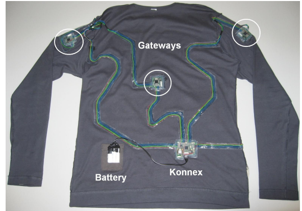
Figure 1: The SMASH (inside out) showing the Konnex and three Gateways (each is marked with a circle, the fourth Gateway is hidden).
