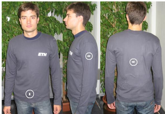
Figure 3: The worn SMASH. White bars at the upper arm, back and lower waist are the Gateway's connectors to Terminals (marked with a circle).
