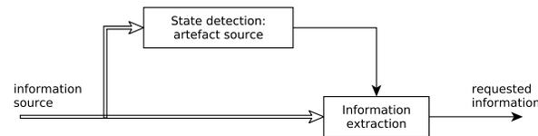
**Figure 2:** Concept of hierarchical artefact compensation
