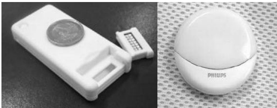
Figure 6: Prototypes of the MyHeart on-body electronics, left: first prototype, right: second prototype (courtesy Philips).
