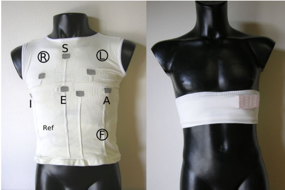
Figure 4: Prototypes of the MyHeart shirt and band textiles (courtesy R. Paradiso, Smartex, Italy). Textile electrode positions are indicated, see text.
